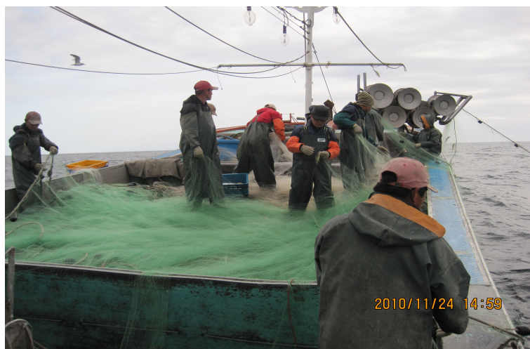
Fig. 3-10. Operating with V-type net hauler of 5 step without the quarter rope.
