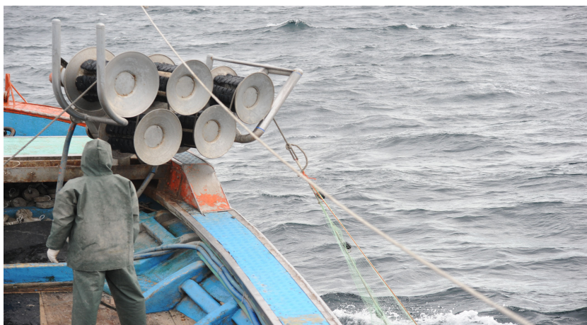
Fig. 3-24. Haul operating of first part of the drift gill net..
