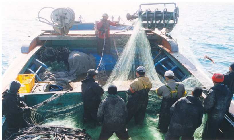
Fig. 3-13. Operating with screw-type net hauler of 4 step without the quarter rope.
