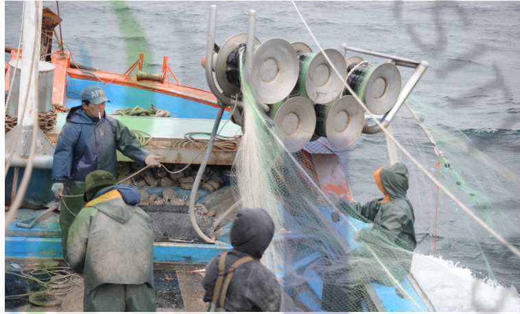
Fig. 3-25. Haul operating by hauler of 5 step.
