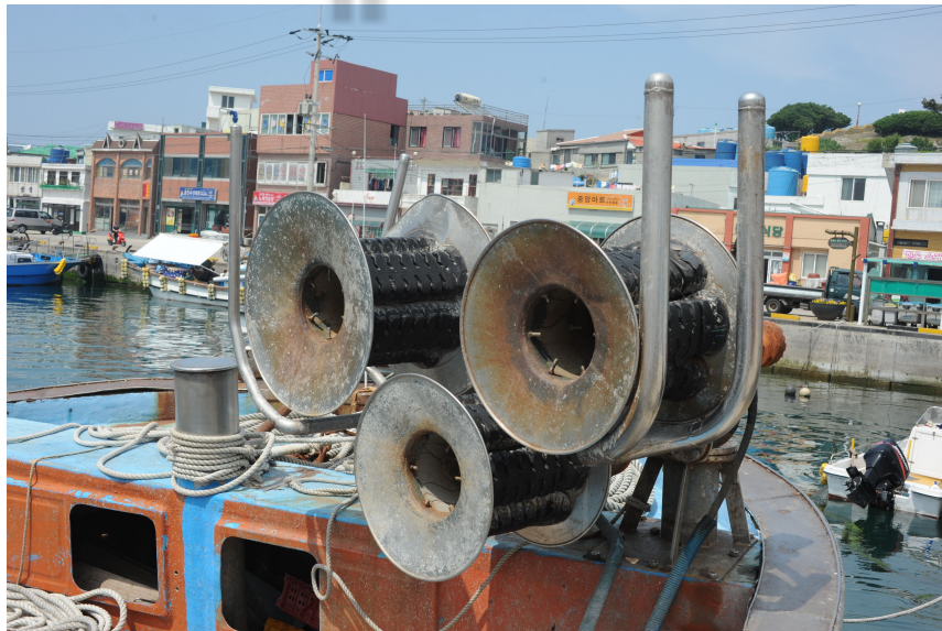
Fig. 3-7. V-type net hauler of 3 step.
