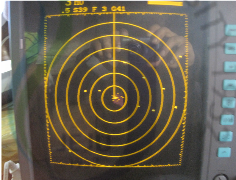
Fig. 3-16. Intervals of fishing boats on radar before casting.
