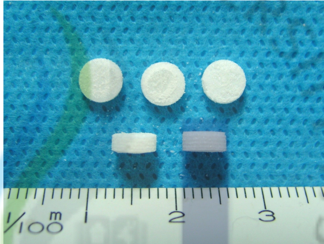
Fig 3. CB1, CB2, CBHA, and CHA implants were shaped cylindrical disks about 5 mm in diameter and 2 mm in thickness and were sterilized by ethylene oxide gas.
