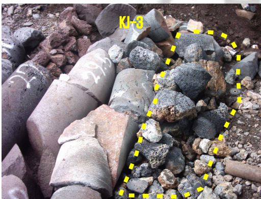
Fig. 17. The hyaloclastite breccia(dotted circle) observed in saline groundwater wells of the eastern area of Jeju Island.
