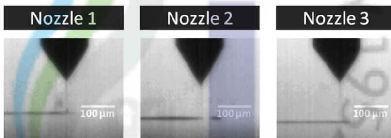
Figure 19 Photographs of axisymmetric liquid menisci established at the nozzle tips of 3ND multi-nozzle EHD inkjet printing head
