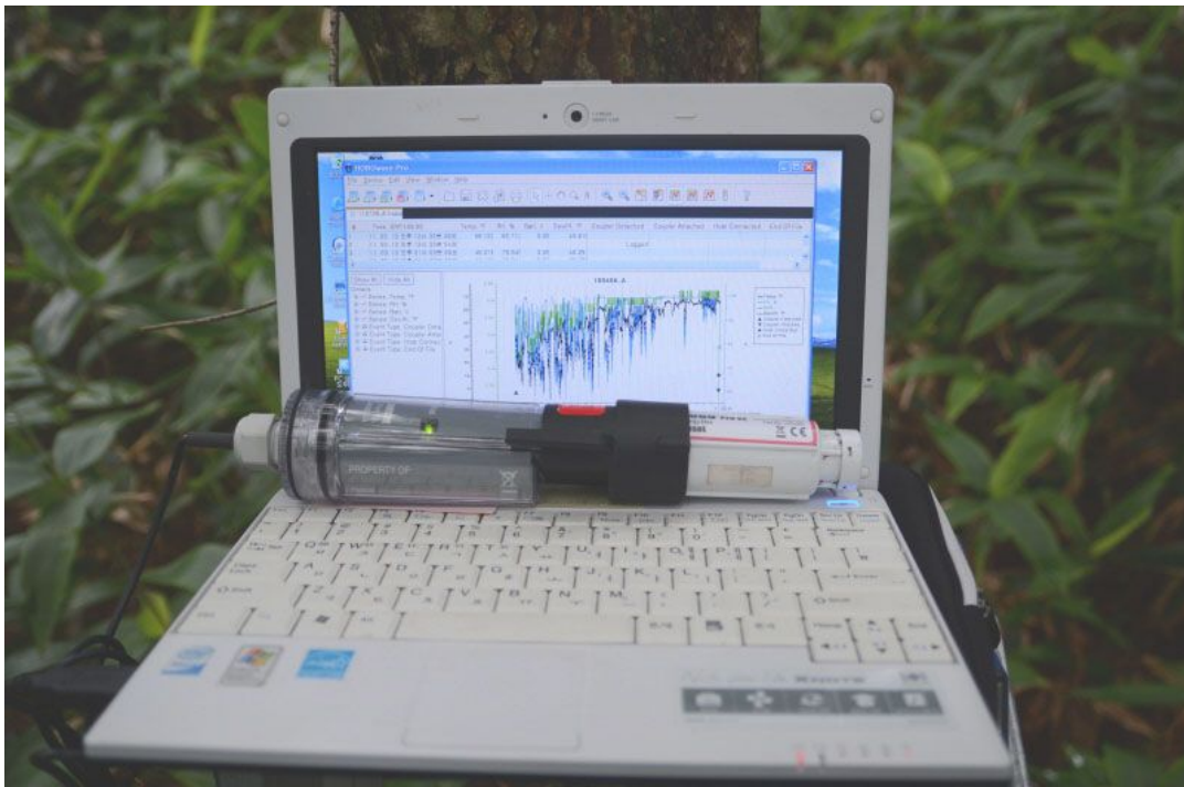
Fig. 2. HOBO : Temperature and humidity logger.
