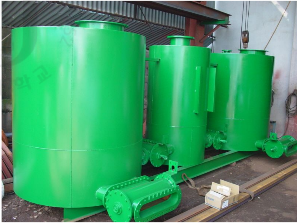
Fig. II-18 Completed compressed air creation device
