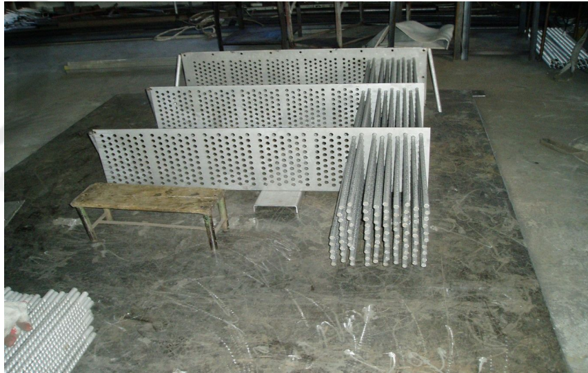
Fig. 6. Fin and tube arrangement heat exchange system (300,000 Kcal/hr) under assembly.
