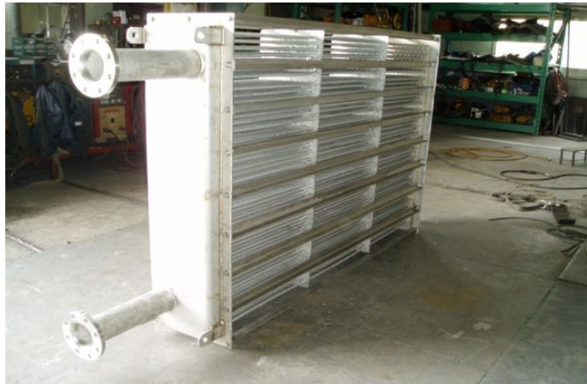
Fig. 7. Photo of the heat exchange system.
