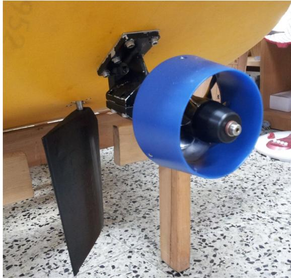
Fig. 29. Thruster mounting
