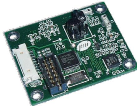
Fig. 40. TCM3(Tilt compensated 3-axis compass module)
