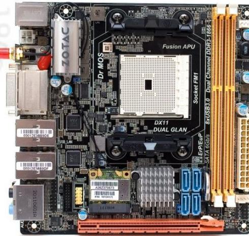
Fig. 34. On-board PC(Zotec Geforce 9400-ITX)
