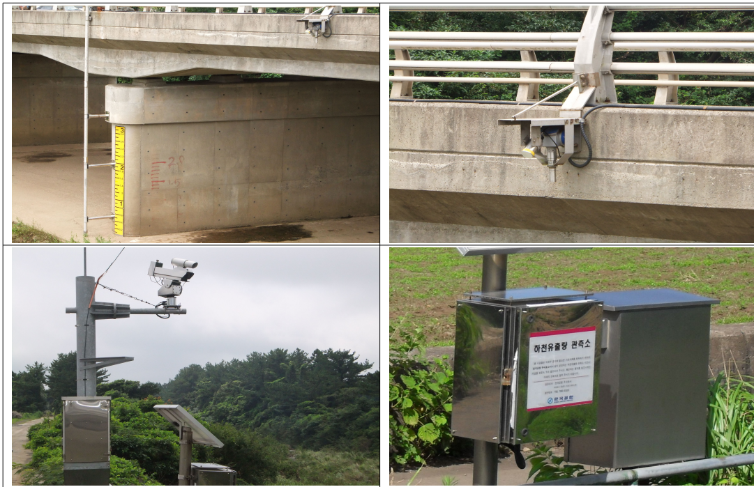
Fig II-4. Water level and water velocity measurement devices
