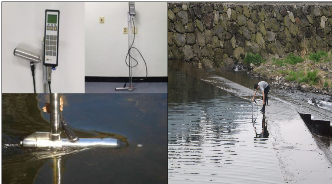
Fig. III-5. Site measurement using ADC
