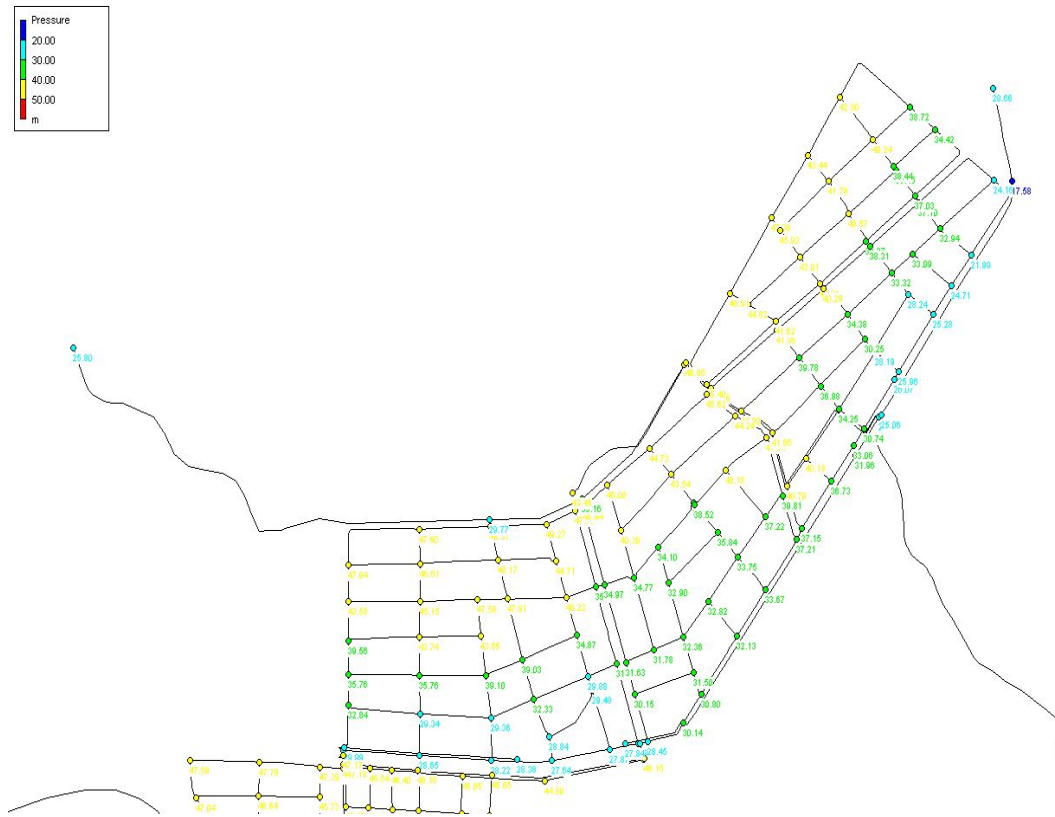
Figure 4.3 Result of pipe network analysis - model 1
