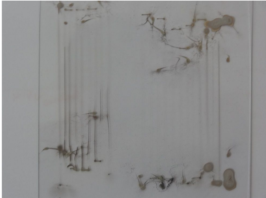
Figure 5.6 Irregular Ag patterns on glass substrate with ParuMicroPE PG-007 using 110 \mu m metallic capillary by applying 5.8kV, after sintering process
