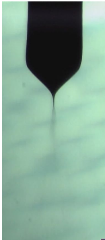
Figure 5.2 High speed camera image cone-jet of Inktec-030 Ag ink at 2.5kV applied voltage and 150 \mu l/hr flow-rate using 110 \mu m internal diameter metallic capillary
