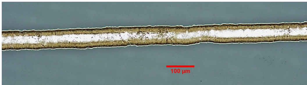
Figure 5.5 Microscope image of Ag pattern using Intech-030, the pattern width is approximately 75 \mu m
