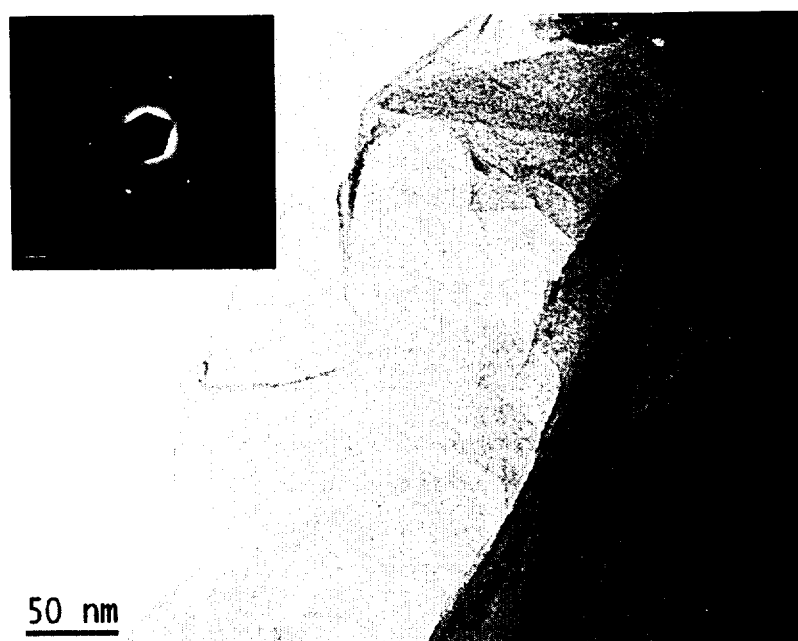
Figure 3.3 High resolution transmission electron microscopic (HR-TEM) image of GO nanosheets. The inset shows the corresponding SAED pattern.
