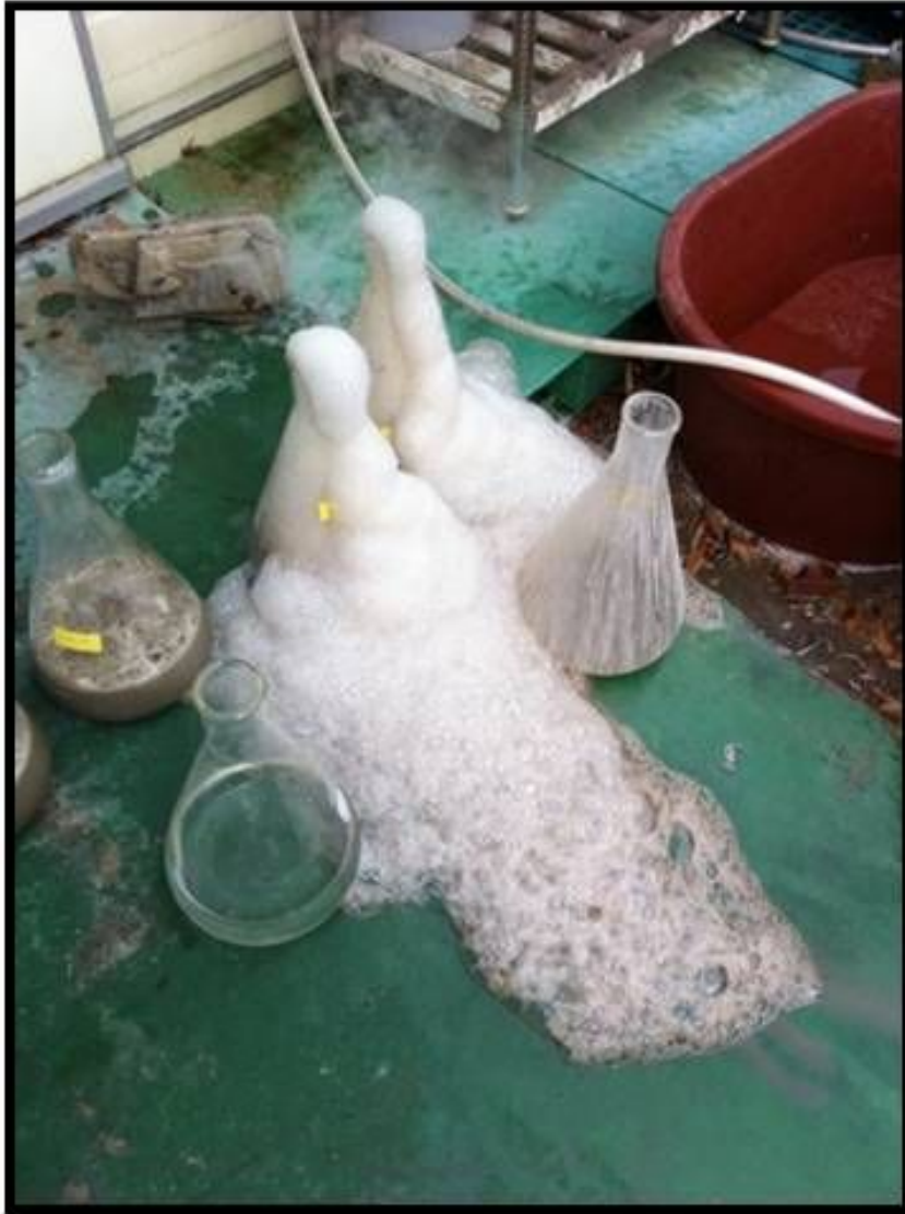
Fig. 2. A pre-treatment of soils. Soil was treated with hydrogen peroxide (10%) for one week.
