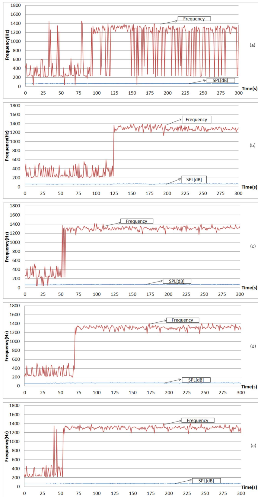
Fig. 21 Frequencies of 50mm resonator tube and stack ; (a) 15mm stack, (b) 10mm stack, (c) 5mm stack, (d) 4mm stack, (e) 3mm stack
