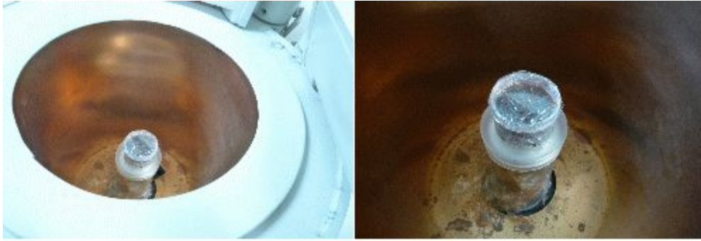
Fig. 18. Is measured using a HPGe (Measuring time: 80,000 sec).
