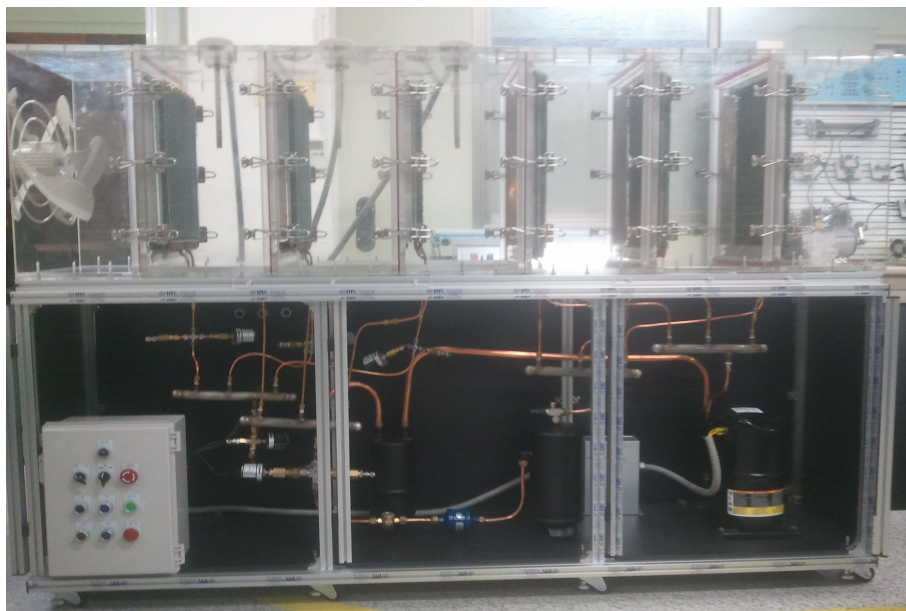
Fig. 4-5 Picture of heat pump
