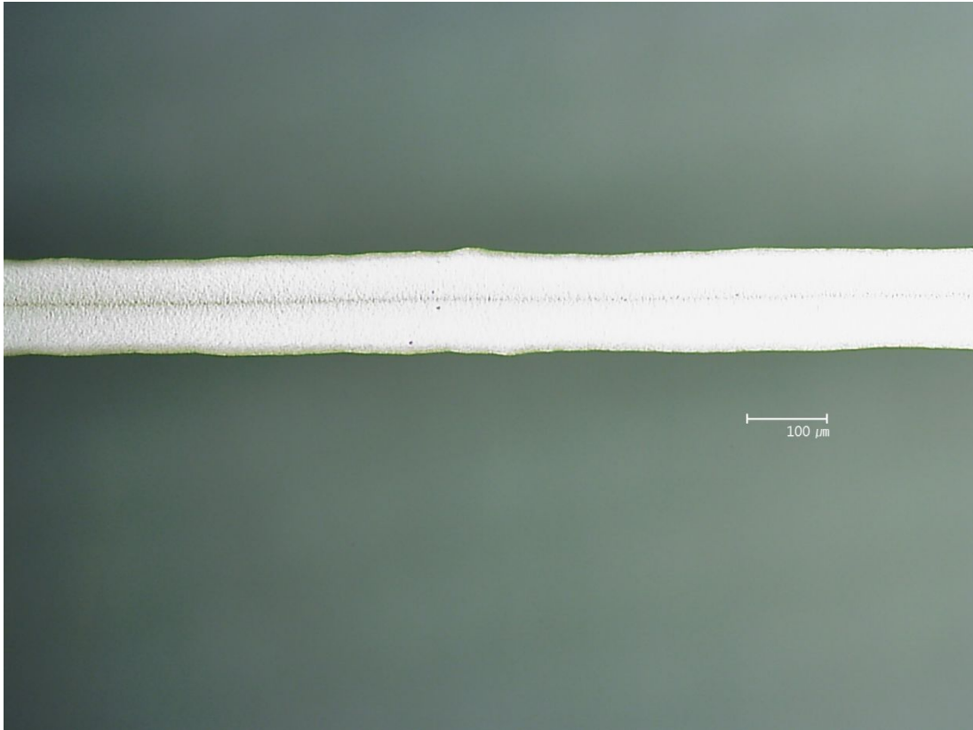
Figure 2.22 Microscopic image of the Ag pattern with a pattern width of around 100 \mu\text{m} .
