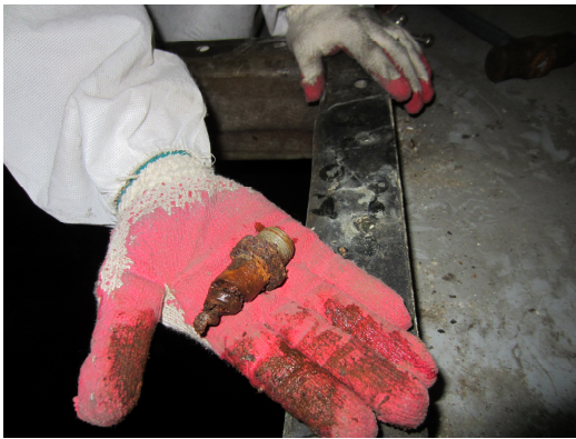
(c) Poor example (clogged spray nozzle)
