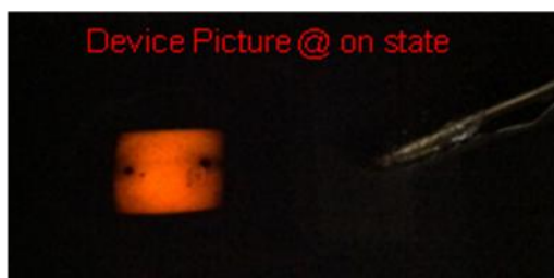
Figure 3-3: Optical Image of the orange light emission from the MEH-PPV based device.
