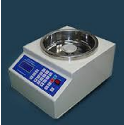
Figure 1-6: Real-time photograph of the Spin coating deposition system and schematic illustration of deposition system.
