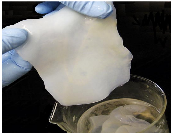
Fig. 1. Bacterial cellulose membrane formed from acetic acid bacteria.
