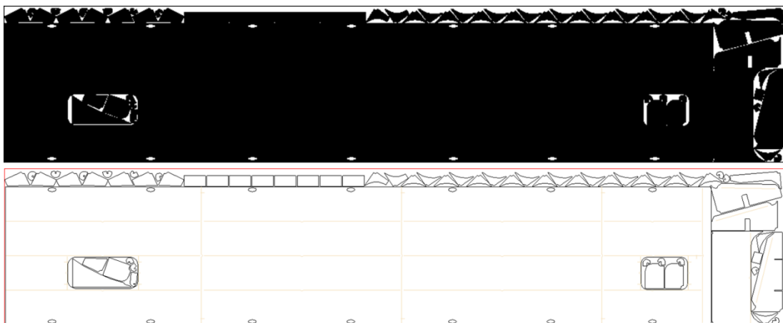
Figure 3.9 Bitmap image (top) and CAD drawing (bottom) from the result of case 2
