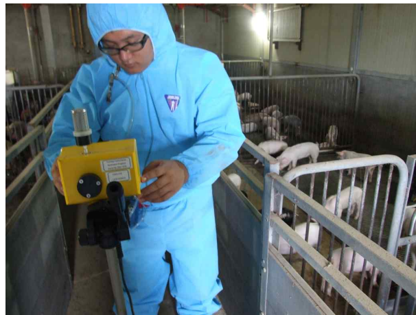
Figure 2. Dust mass concentration measurement in swine facilities.
