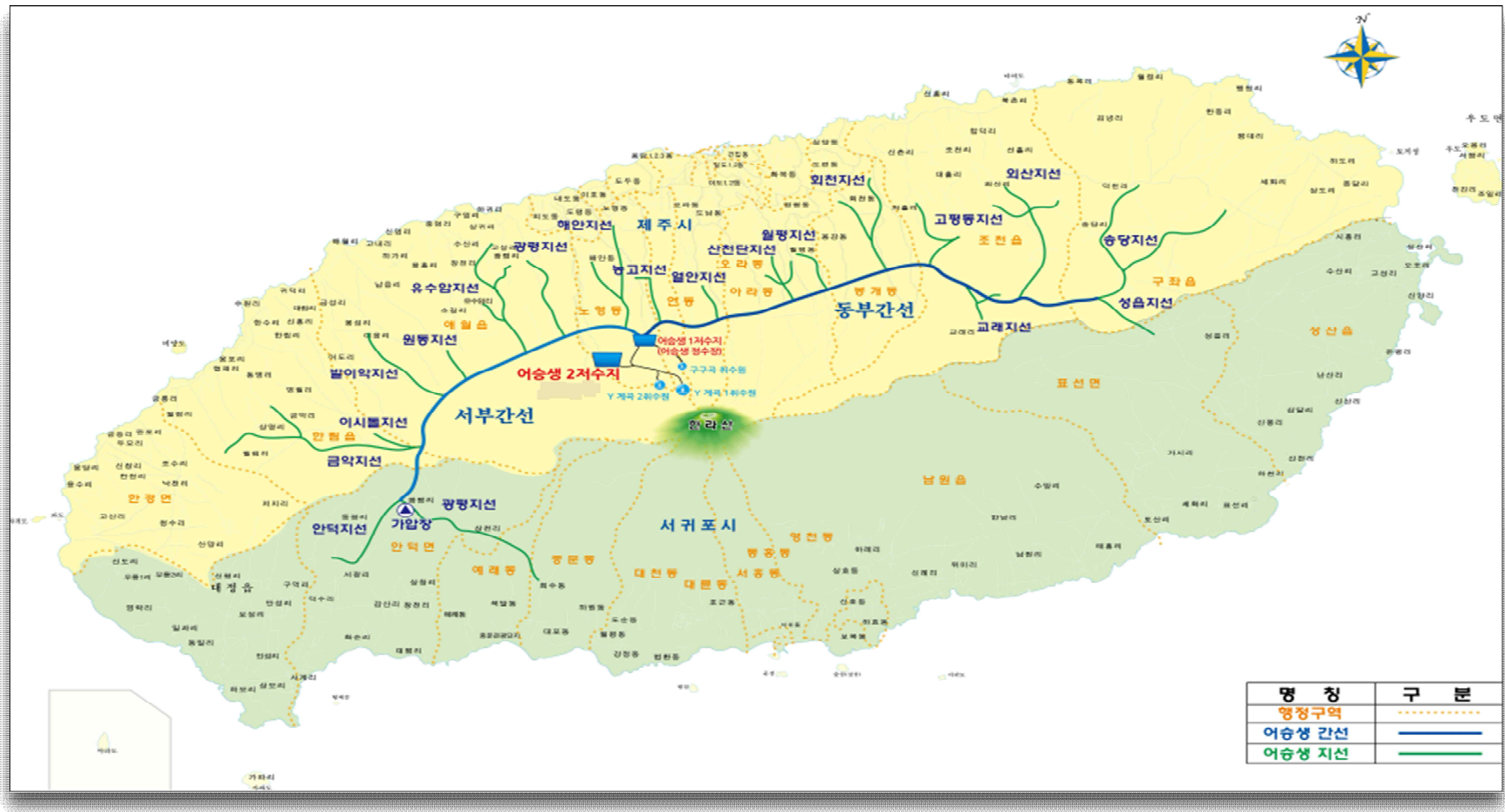
Fig 1. Water treatment plant Eoseungsaeng pipe network.
