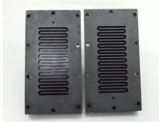
Fig. 10. The flow channel structure of the cell.
