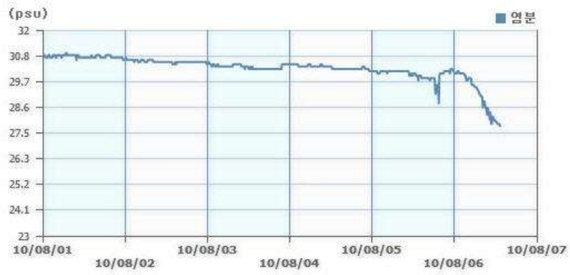
<Fig. 43> Time series of salinity observed at Chu-ja island. Salinity drastically decreased from August 6, 2010.
