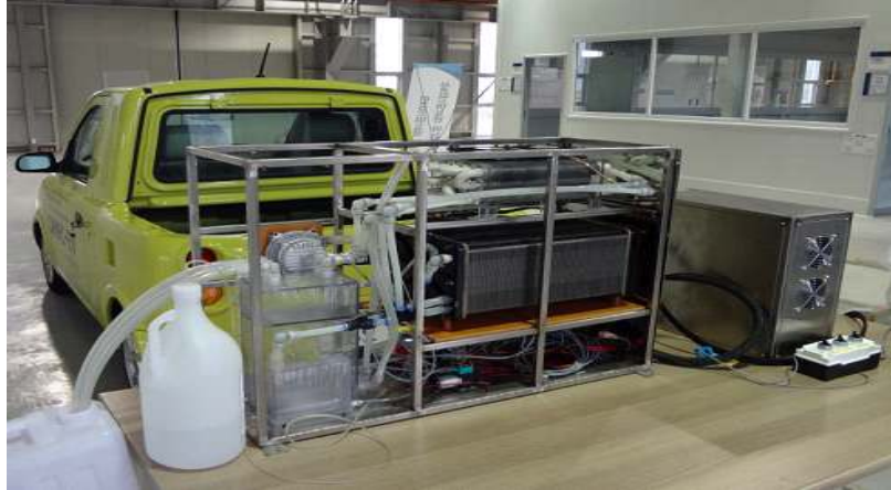
Fig. 21 2 kW class DMFC control system
