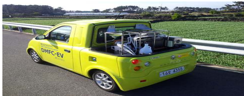
Fig. 7. Electric vehicle system with the 2 kW class DMFC in CHANGE
