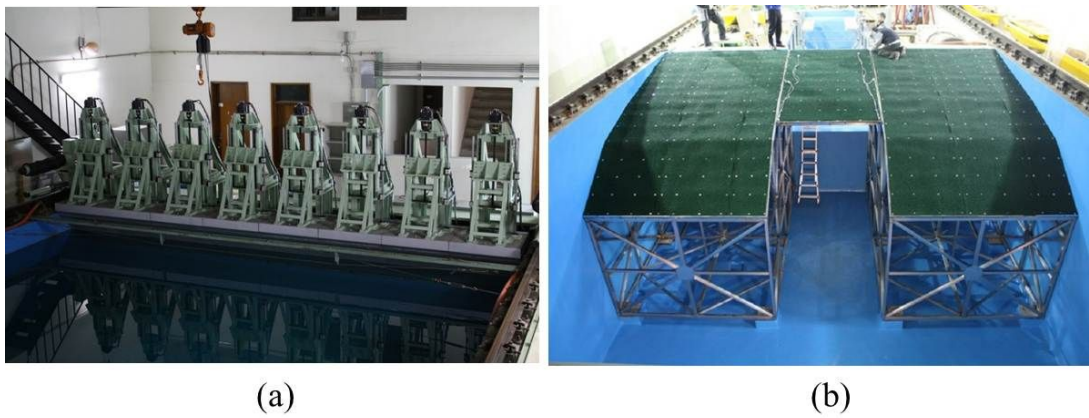
Fig.3.14.Wave generating system of the SNU wave tank.(a) plunger-type wave maker, (b) beach-type wave absorber.
