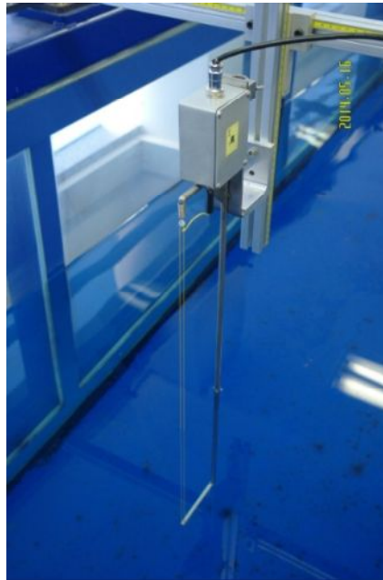
Fig.3.11.Capacitance-type wave gauge installed on the JNU wave tank.
