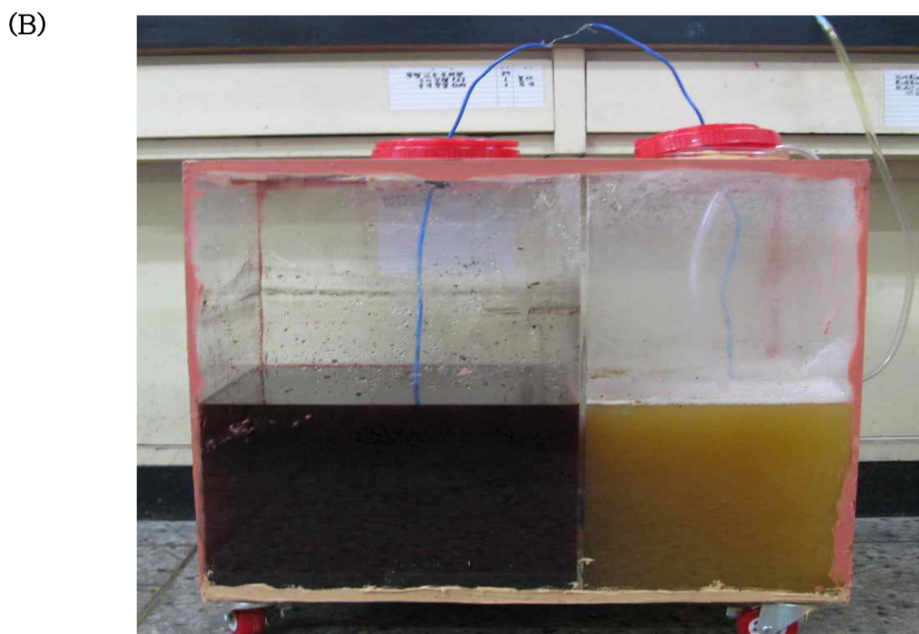
Fig. 3. Microbial fuel cell constructed in this study.
