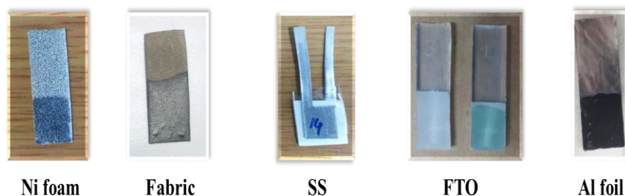
Figure 2.1.1 Fabricated binder and binder free electrodes on various current collectors.
