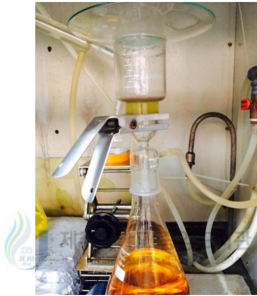
Figure 11. Process to filter the soil samples.
