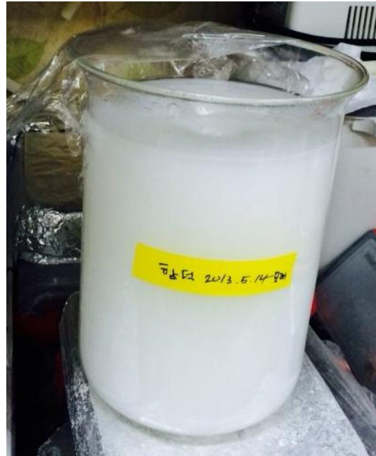
Figure 14. Carbonate precipitation process of sand samples.
