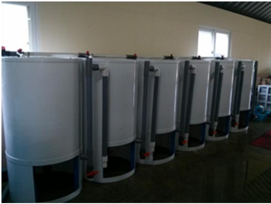
Figure 4-1. Feces collection tanks (Guelph system) used for the apparent digestibility test of citrus by-product containing diets.
