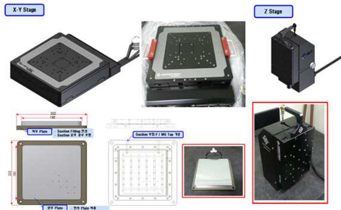
Fig. 8 Sunction plate design for X-Y-Z micro transfer stage shaft and substrate fixing
