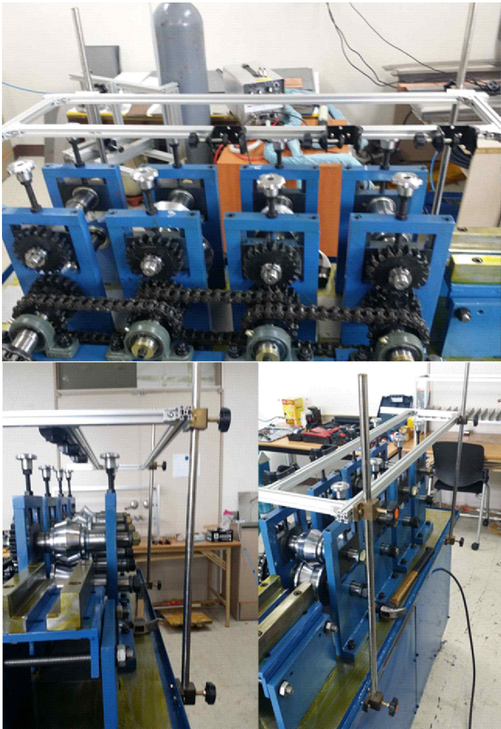
Fig. 31 Apparatus for pre-heating in roll forming machine
