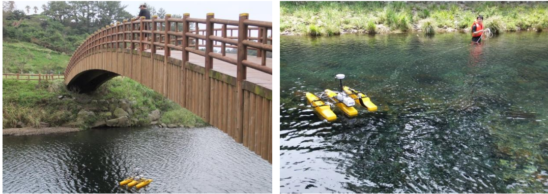
Fig. 3.7 Site application photo of ADCP for discharge observation
