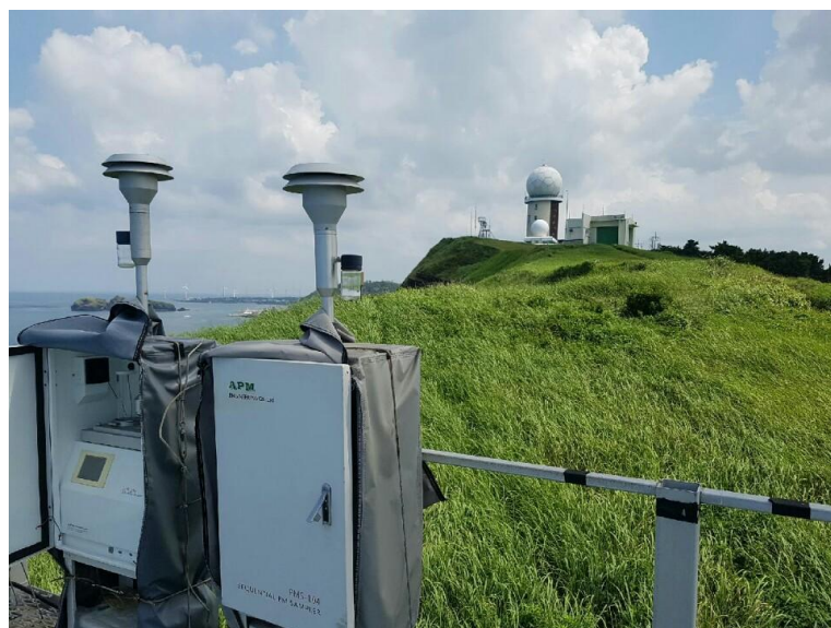
Fig. 2. PM_{10} sampler (APM Engineering, PMS-103, Korea).
