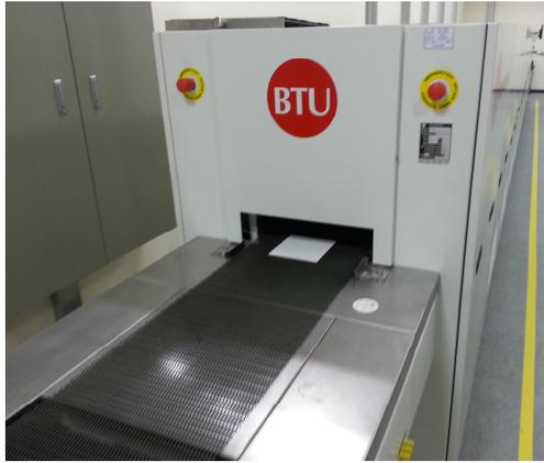
Fig. 55. Sintering furnace.
