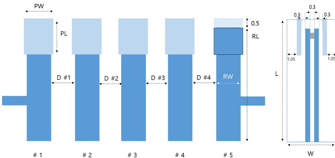
Fig. 28. LTCC filter structure for WCDMA band.
