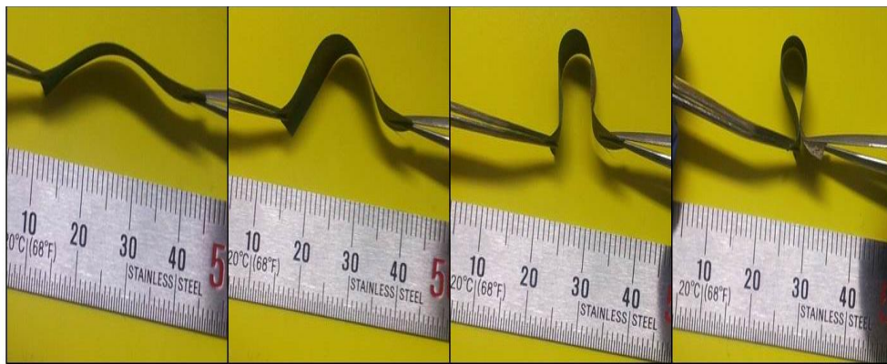
Figure 7.1.13 Photographic images of flexibility of the deposited \text{CoMoO}_4@ \text{Co}(\text{OH})_2 on conductive textile at the different bending conditions.
