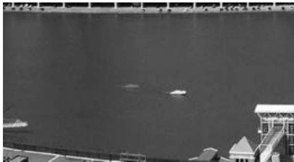
Fig. 8. Stitching result of acquired image (After-image (ghost phenomenon))
