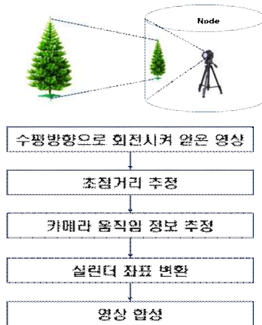
Fig. 21. Cylinder panorama construction principle and Flow Chart
