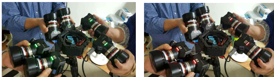
Fig. 41. Simultaneous recording signal Ready (greent) and ready Recording status after the simultaneous recording signal (red)
