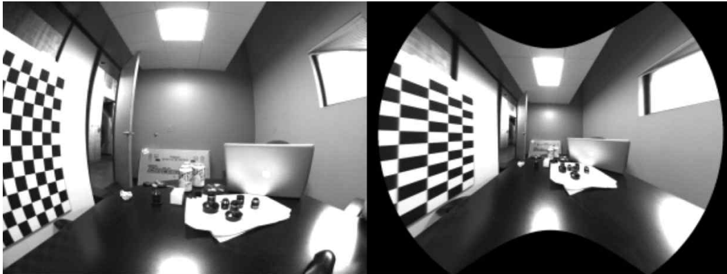
Fig. 33. An example of raw image with lens distortion and its correction
