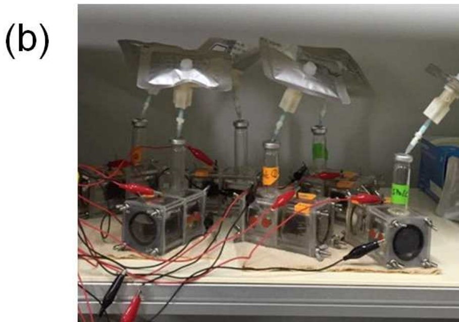
Fig. 5. (a) Generalized schematic diagram of microbial electrolysis cell (MEC), showing two chambers separated by an anion exchange membrane (AEM) with the voltage set using a power supply. (b) Two chamber MECs used in this research.
