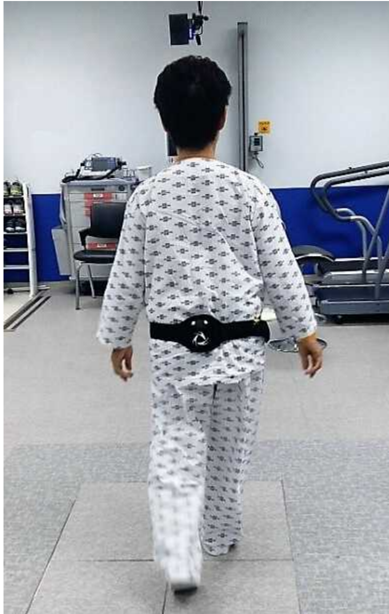
Figure 2. The figure shows spatiotemporal gait analysis using a validated 24 wireless inertial sensing device (G-Walk ® , BTS Bioengineering S.p.A., Milan, Italy)
