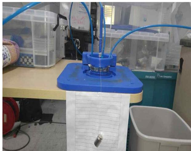
Fig. 7-11 Experimental apparatus for measuring mechanical power of Gadolinium generator
