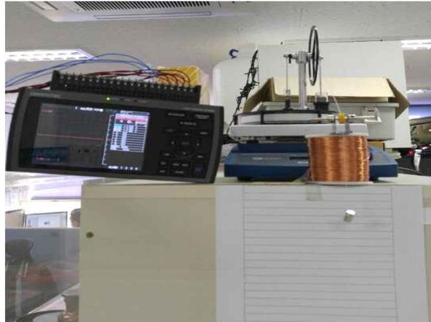
Fig. 7-3 Experimental setup for mechanical power measurement
