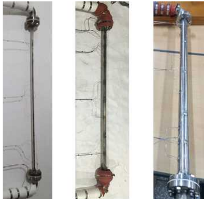
[Fig. 11] JNU condenser tubes with different diameters
