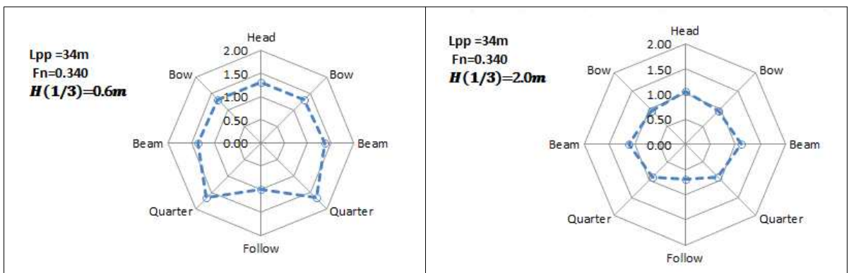
Fig. 11 GM fluctuations with respect to waves components= 0, 045, 090, 135, 180°at ship speed 12kn'ts, Beaufort scale No. 3 and 5
