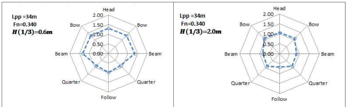
Fig. 12 GM fluctuations with respect to waves components= 0, 045, 090, 135, 180°at ship speed 12kn'ts with 1kn'ts current Beaufort scale No. 3 and 5
