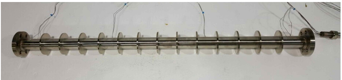
Fig. 3-25 Photograph of the fabricated annular finned tube.
