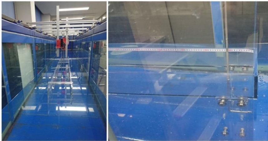
Fig. 3.6 Photograph of a water channel resonator installed in wave tank and a wave gauge installed at wall
