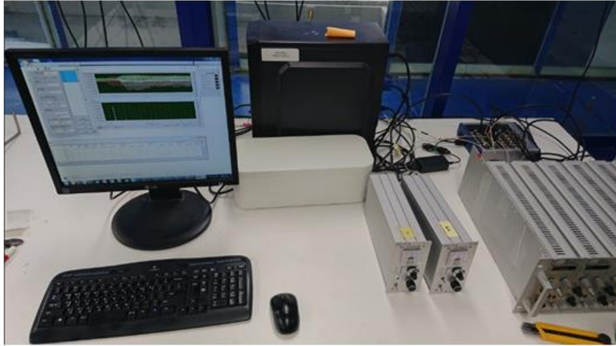
Fig. 3.3 Measurement systems(Computer, DAQ board, amplifier)
