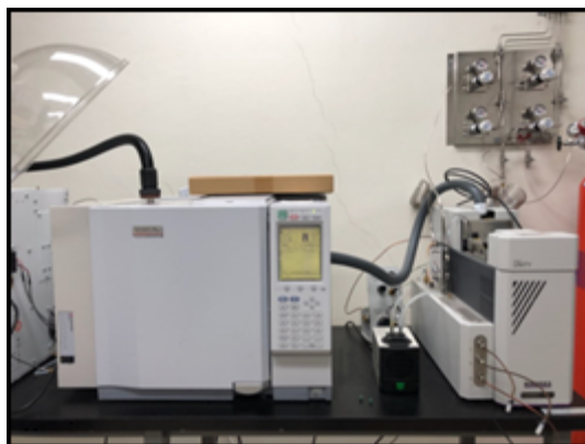
Figure 2. Gas Chromatograph equipped with Flame Photometric Detector.
