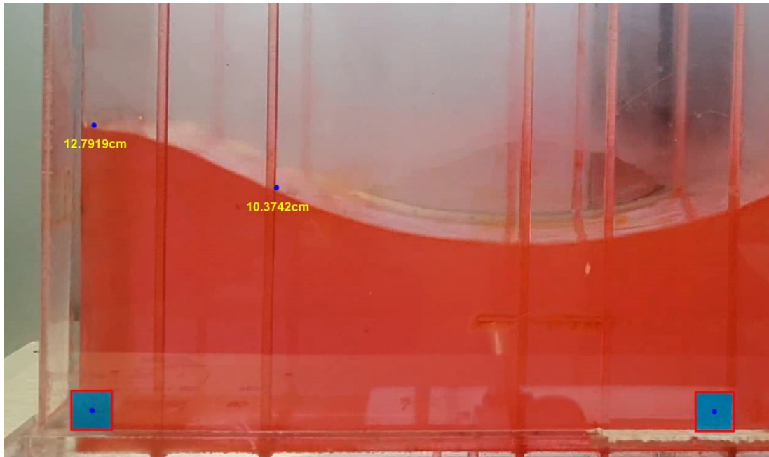
Fig. 2-8 Snapshot of the Image tracking for measuring water elevation and tank motion
