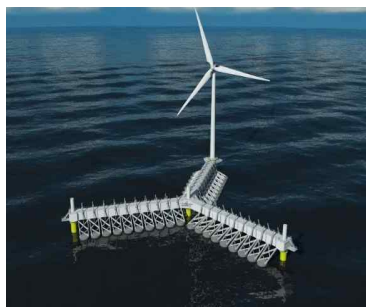
(c) Hybrid system(Wave Star)
