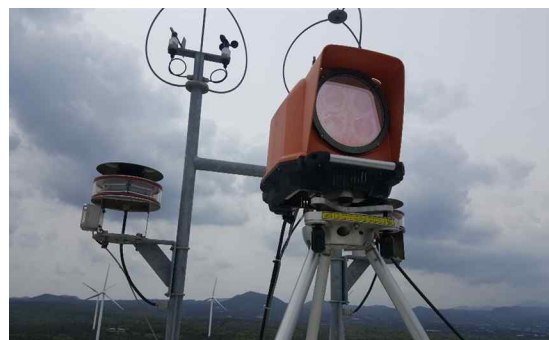
<4-beam nacelle LiDAR installed on Dongbok wind turbine no. 1 (photograph by D. H. Shin)>
