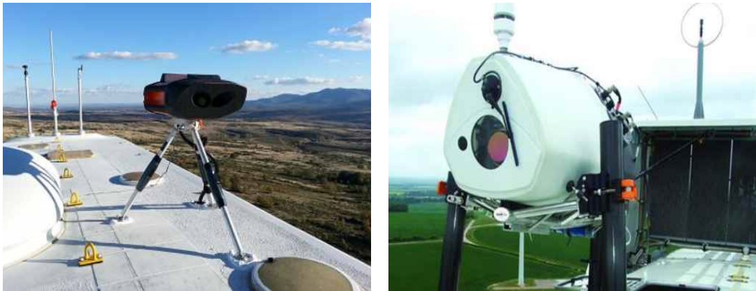
Fig. II-2 Example of a nacelle LiDAR [85, 86]
