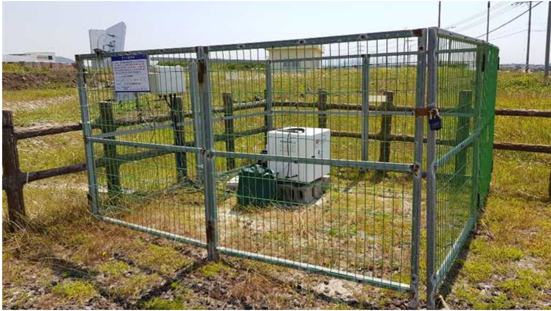
<Ground LiDAR installed in Haengwon wind farm (photograph by D. H. Shin)>
