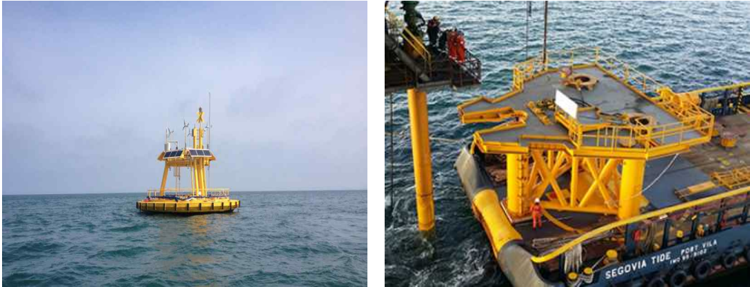
Fig. II-4 Example of floating and platform LiDARs [89, 90]
