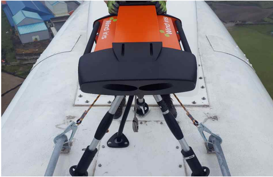
Fig. III-6 2-beam nacelle LiDAR on a test wind turbine at the Haengwon wind farm
