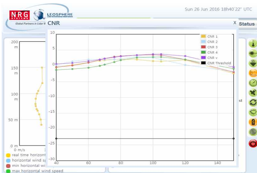
Fig. III-13 Real time monitoring of CNR signals from the ground LiDAR
