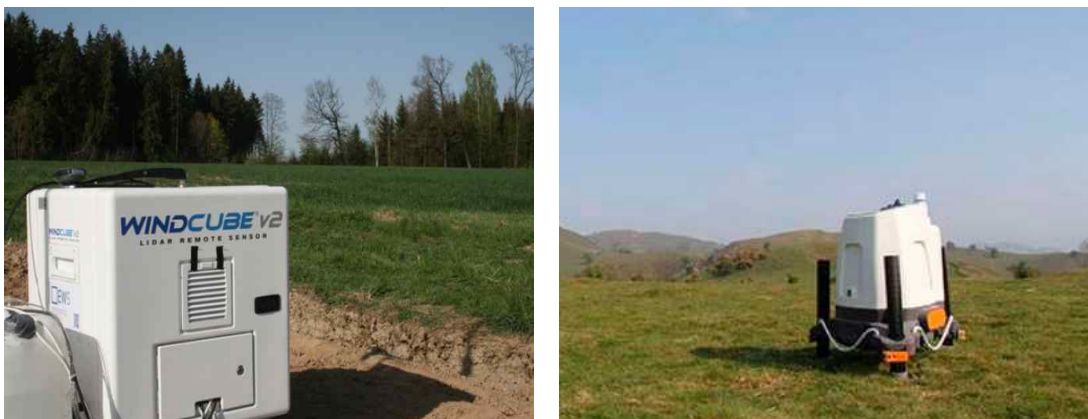
Fig. II-3 Example of a ground LiDAR [87, 88]
