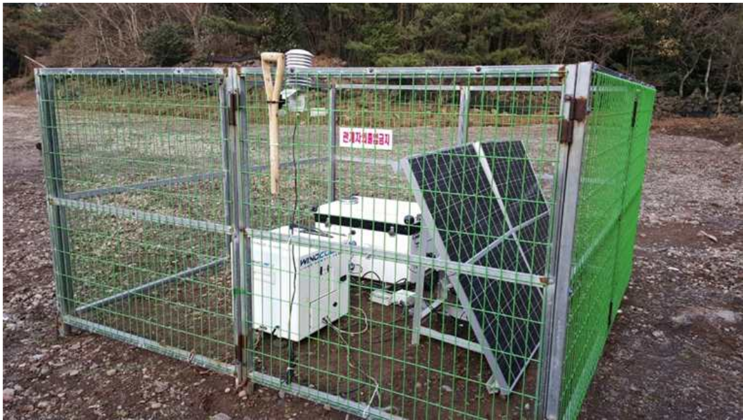
<Ground LiDAR installed in Dongbok wind farm (photograph by D. H. Shin)>
