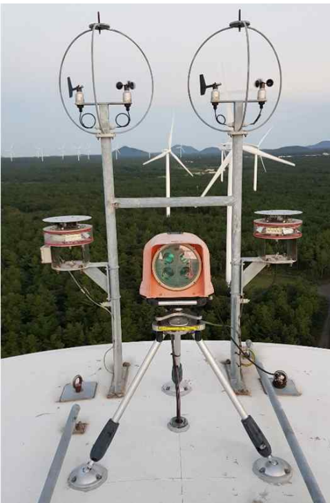
<4-beam nacelle LiDAR installed on Dongbok wind turbine no. 1 (photograph by D. H. Shin)>
